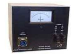
Ohm-Labs KV-R is a portable precision dc high voltage divider for measurement up to 10 kV.
